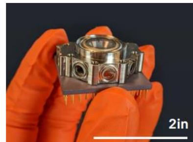
An IonQ ion trap and vacuum chamber
